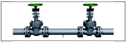
The age-old "Double Block & Bleed" system (as shown above) required the use of two valves and a spool piece. A bleed valve was used to drain the spool and verify seal integrity.
