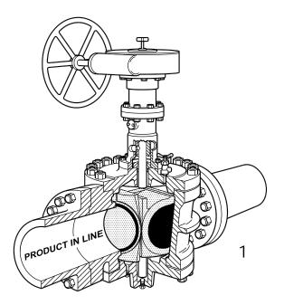
You can forget about line draining, line flushing, vacuum trucks and product losses - General's Twin Seal Seat and Reseat valve eliminates them all.
