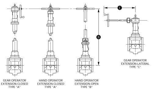
General Twin Seal makes both vertical and lateral extensions or combinations of both.
