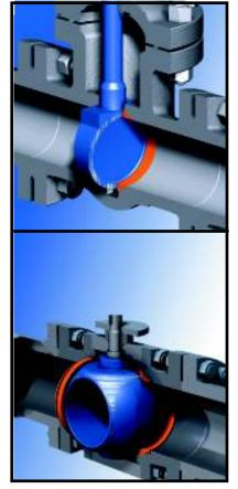
Scored seating segments Seal abrasion is inherent in the design of most ball and gate valves. In most instances, the seats are ground or wedged against metal every time the valve cycles. Any foreign material lodged between the seats and ball or gate will score the seating surfaces. Once the seating segment is scored, product loss and contamination results. The General Twin Seal avoids abrasion by having both independent slips totally retracted from the body bore during cycling.
