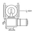
Style "A": Actuator mounted parallel to pipe line.
