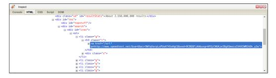
Here, we see that the search results are structured as links whose parent element is a <h3> tag of class "r". To scrape the search results we will use a CSS selector, which were introduced in *Chapter 2, Scraping the Data*:
