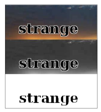
The text in the final thresholded image is much clearer and is ready to be passed to Tesseract:
