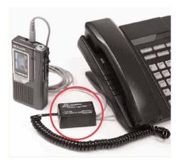
To record audio in rich media files, such as audio and video files, you must use a phone recording adapter that supports bi-directional audio between your phone and computer—that is, connects to both the input and output jacks for your computer's sound card. The DynaMetric TMP-636 adapter supports bi-directional audio.
