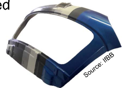
Tailgate made from various natural and carbon fiber-reinforced epoxy
