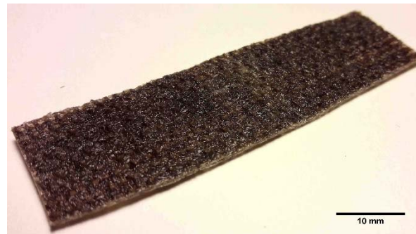
Flax fabric, coated with diluted epoxy resin
