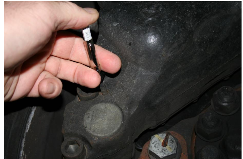
Pad wear indicator measurement using a tire tread depth gauge
