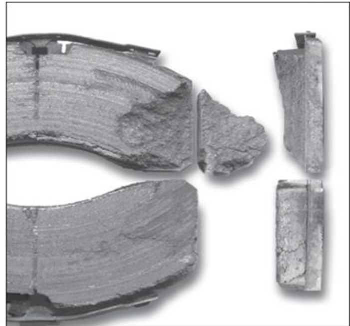
Brake pads showing unacceptable wear—note edges
