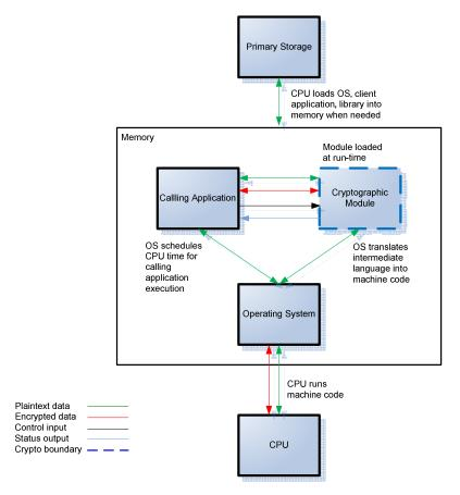
Figure 2 - Logical Block Diagram and Cryptographic Boundary
