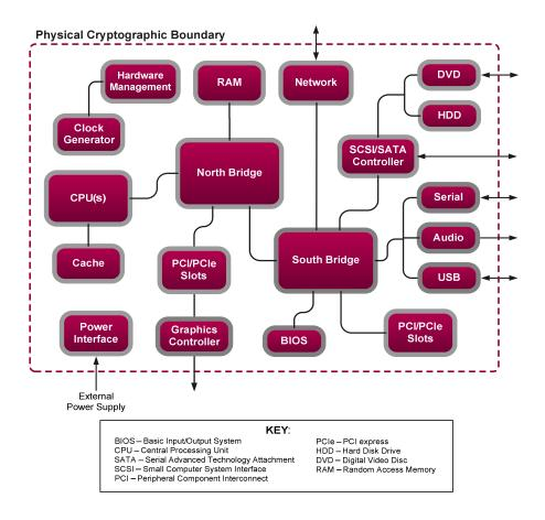
Figure I - V-Series Appliance Hardware Block Diagram
