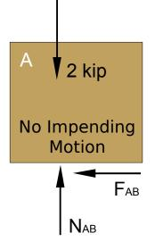
Construct a FBD of wedge B. Motion is to the left, so the force of friction is to the right and parallel to the bottom surface. The weight of Block A is shown as N<sub>AB</sub>. By similar triangles, angle θ is 7°.
