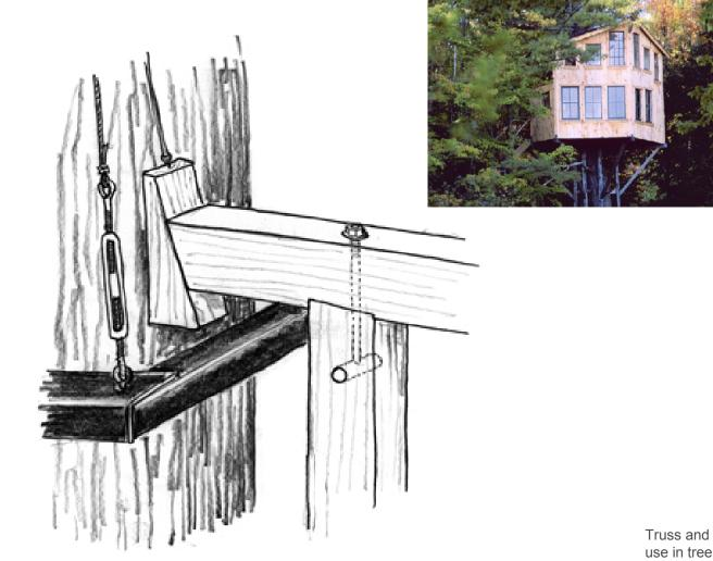
Truss and Collar Wedge detail for use in treehouse construction
