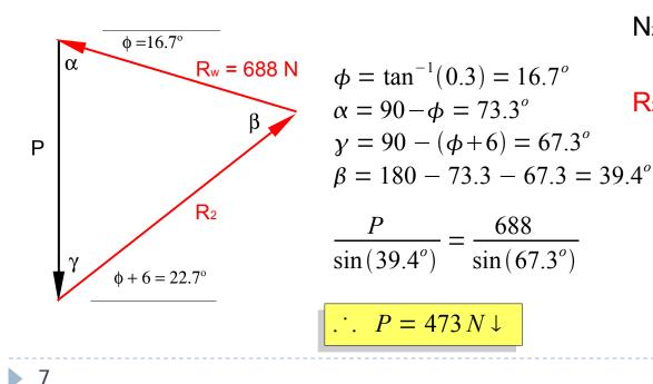
Determine the smallest values of forces P<sub>1</sub> and P<sub>2</sub> required to raise Block A while preventing Block A from moving horizontally. The coefficient of static friction for all surfaces of contact is 0.3. The weight of wedges B and C is negligible compared to the weight of Block A.
