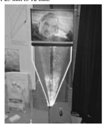
Fig. 20: Image projected via a 25 mm thick acrylic light-guide
