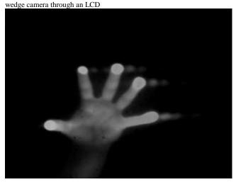
Fig. 23: A hand touching the screen, imaging at infra-red wavelengths with a wedge camera through an LCD (uses a leaky front light diffuser)
