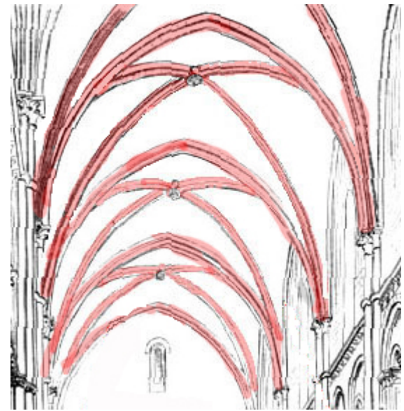
Ribbed groin vault
