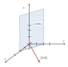
Note that the [110] direction is normal to the (110) plane. **The angle is 90 degrees.** In general, one can prove that a [hkl] direction is normal to an (hkl) plane.
