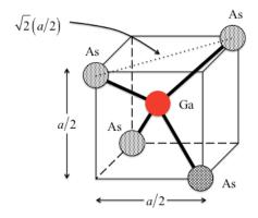
If the atom in the **upper left** of the sub-cube is As, then the nearest neighbor is the Ga atom in the center of this sub-cube. The nearest **As atom** is the one on the top face center of the big cube or the one at the **back right** of the sub-cube shown above. The distance is
