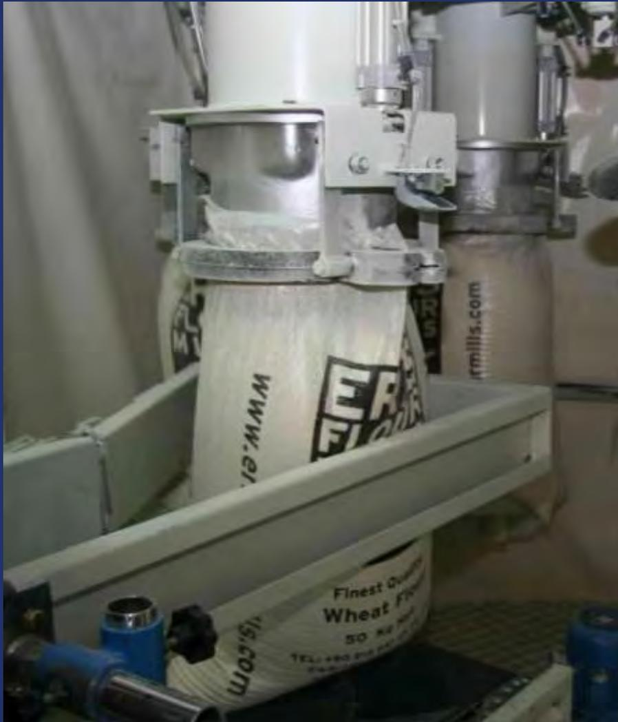
The filled bag is placed onto a belt conveyor.
