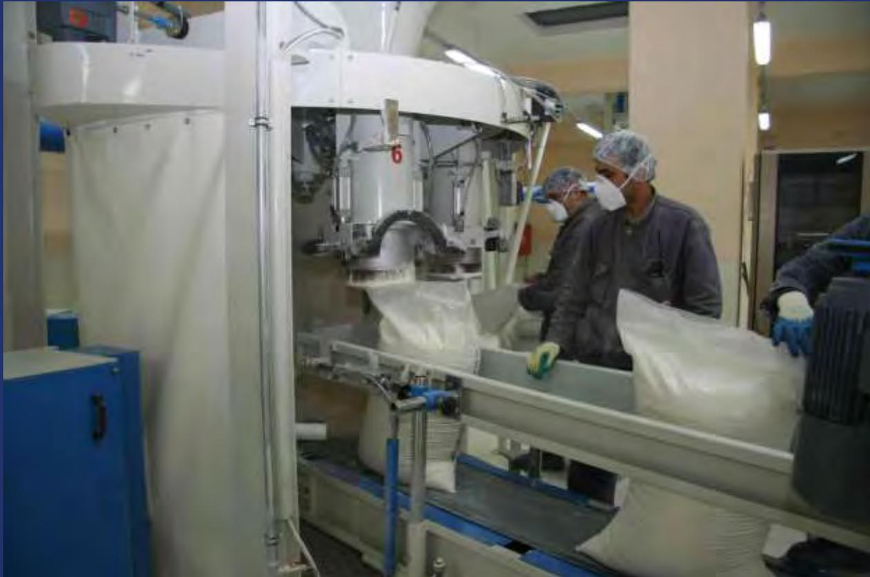
The bag is transferred in upright position into the bag closing device.
