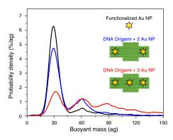
**Fig. 5.** Buoyant mass measurements of DNA origami–gold nanoparticle assemblies. Buoyant mass distributions (kernel density estimates) of functionalized 15-nm gold nanoparticles (Au NP) with ssDNA (black) mixed with DNA origami structures with two binding sites (blue) and DNA origami structures with three binding sites (red).
