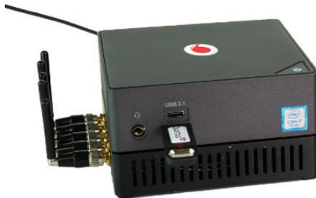
LimeNET Mini For Indoor Base Station test as “crowdcell” and as UE
