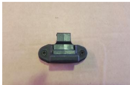
Fig.19 - Nylon Striker Plate Alwin Rear Door
