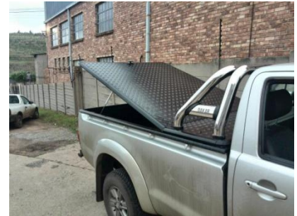
*Alwin LDV Aluminium Lid Cover with gasstays
