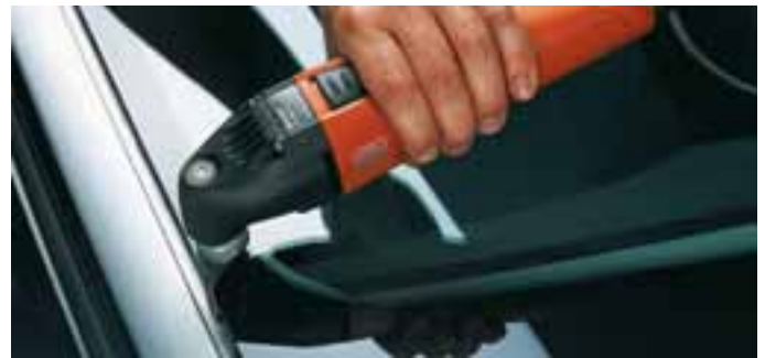
The essential tool for removing rigidly bonded windshields – the FEIN SUPERCUT AUTOMOTIVE.
