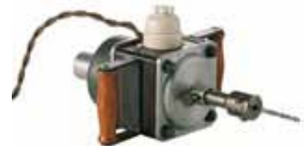
The first electric handheld power drill built with aluminum components. Built in 1900.
