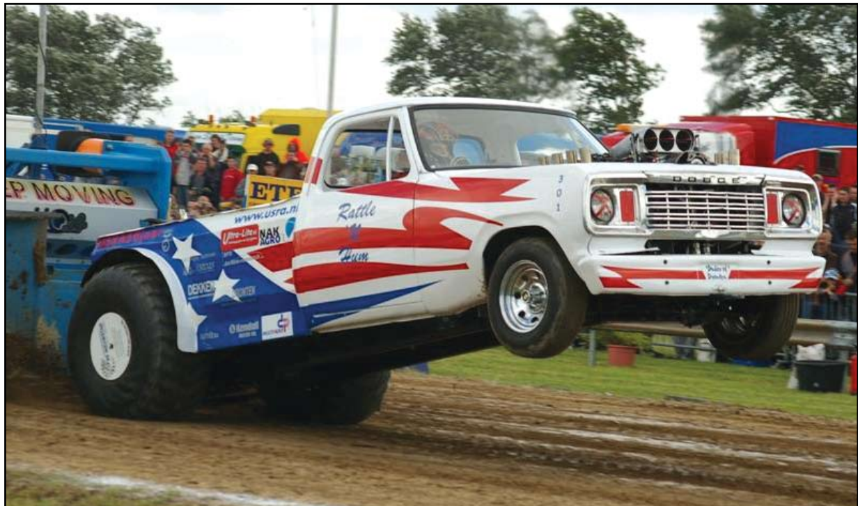
Team Rattle'n Hum / BFS Martin Wolters. The Worlds only Two Wheel Drive Tractor Pulling Team by students of Agricultural High School Dronten in Holland. Uses Ferrea Titanium Intake and Exhaust Valves in the 500 cu. Blown Big Chief engine.
