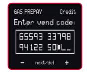
Using the + and - buttons, add the vend code. Press Next to go to next number, or touch and hold to delete/correct an error
