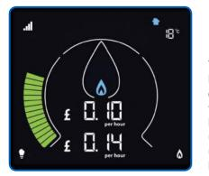
Your current usage is displayed on the left hand side of the Home screen. The outer gauge shows your electricity, and the inner flame your gas. Gas usage may take a bit longer to update – up to 30 minutes. You can use the touch-sensitive unit selectors to view your usage in pounds and pence, kilowatt hours (kWh), or carbon emissions.
