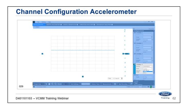
This screen appears when you place the Accelerometer in one of the channel ports.
