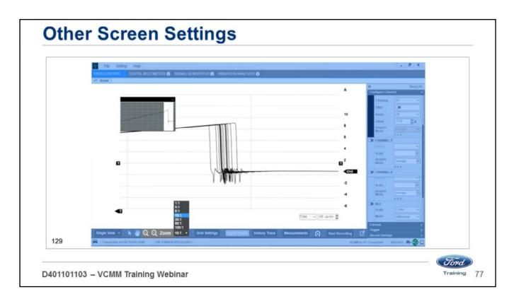
The Zoom feature allows you to zoom-in on a subset of a scope frame without having to change the data acquisition configuration.
