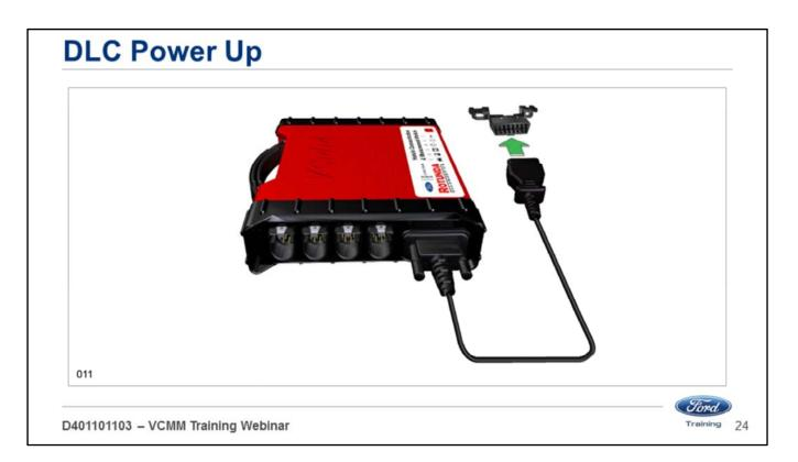
• Connect the 16-pin end of the DLC cable to the vehicle DLC.
