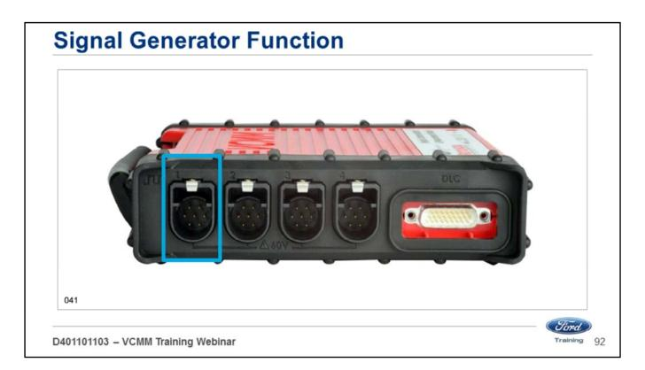
You can only choose channel 1 when using the signal generator function.
