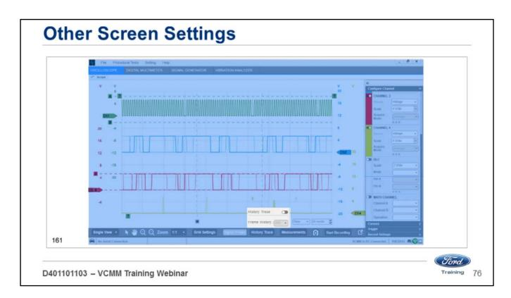
The channel trace history feature is accessed using the Control Bar's History Trace button. This feature retains a history of channel traces, up to a specified maximum.
