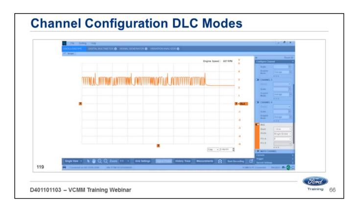
Single ended mode allows you to monitor any of the 16 pins in the DLC except pins 4, 5 and 16.
