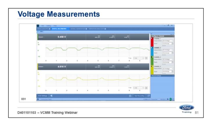
To measure DC voltage place the test probe in one of the four channels and choose DC Voltage from the drop-down menu:
