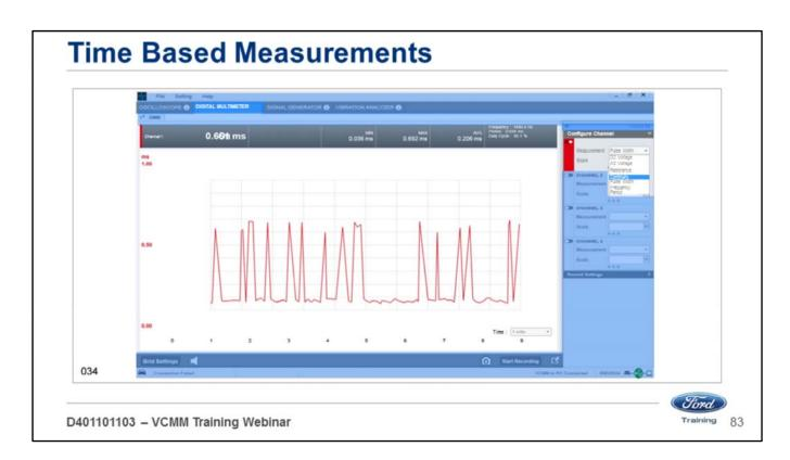
To make time based measurements place the test probe in one of the four channels:
