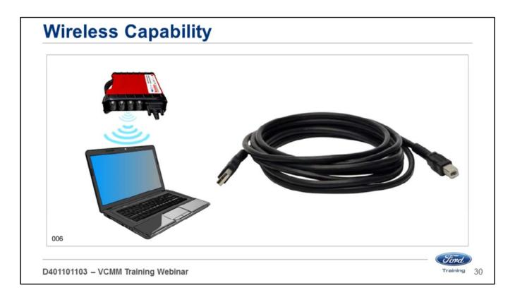
The following procedure describes how to connect your VCMM to the PC using the preferred method of point-to-point wireless communication.
