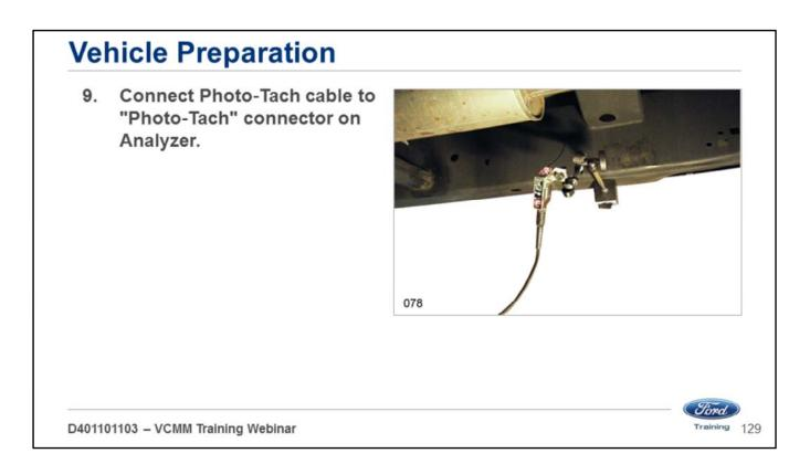
9. Connect the Photo-Tach cable to the Photo-Tach connector on Analyzer.
