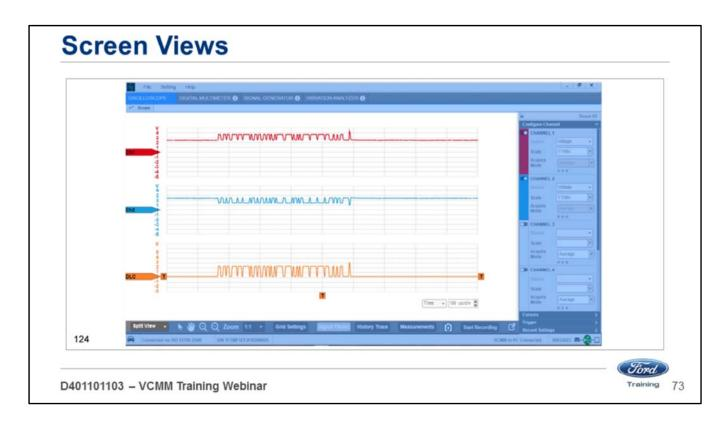
In split view you can separate the signals – CAN Hi/CAN Low in a CAN circuit.
