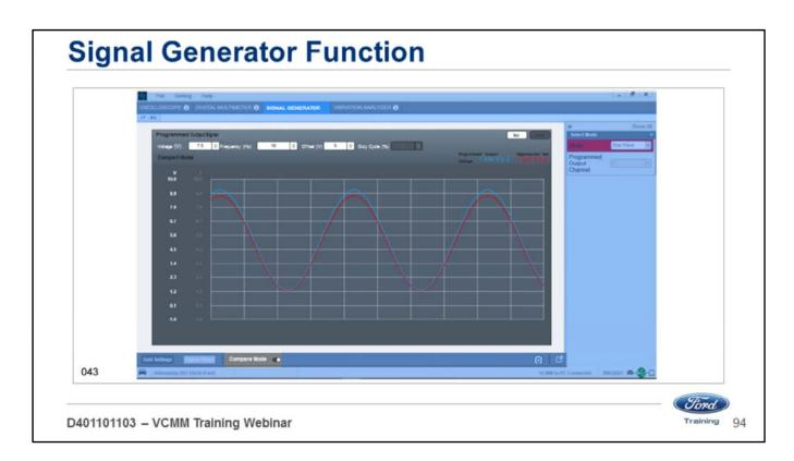
Here is the same sine wave signal at 7.5 volts and 10 hertz in the compare mode.
