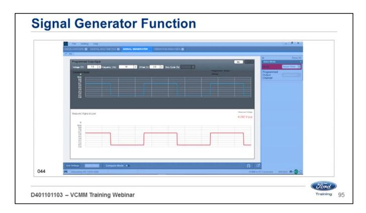
Here is an example of a square wave signal at 7.5 volts and 10 hertz.
