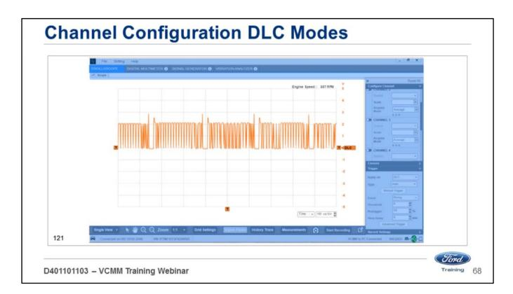
Differential mode allows you to monitor the voltage differences between any 2 of the 16 pins in the DLC except pins 4, 5 and 16.
