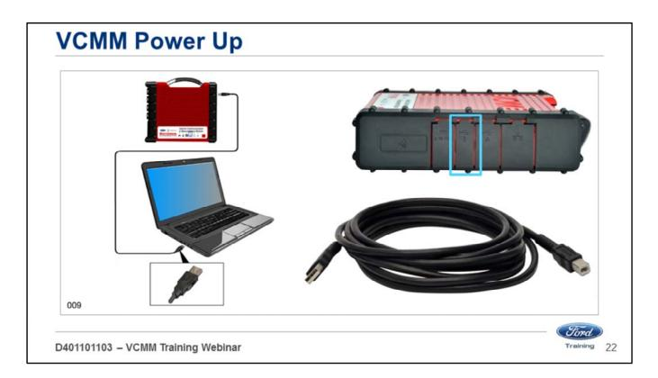
Connect the type A end of the USB cable to the PC USB port.
