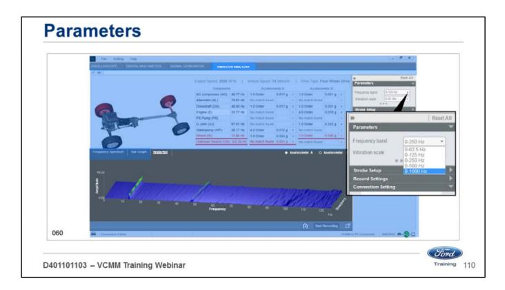
You can change the frequency band parameters from 0-62 Hz to 0-1000 Hz.
