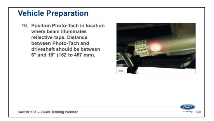
10. Position the Photo-Tach in a location where the beam illuminates the reflective tape. The distance between the Photo-Tach and the driveshaft should be between 6" and 18" (152 to 457 mm).
