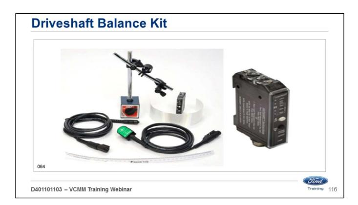
To balance drive shafts you can use the kit shown above.
