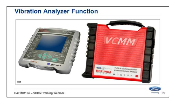
The VCMM has all of the vibration analyzer functionality of the Vetronix MTS 4000/4100.
