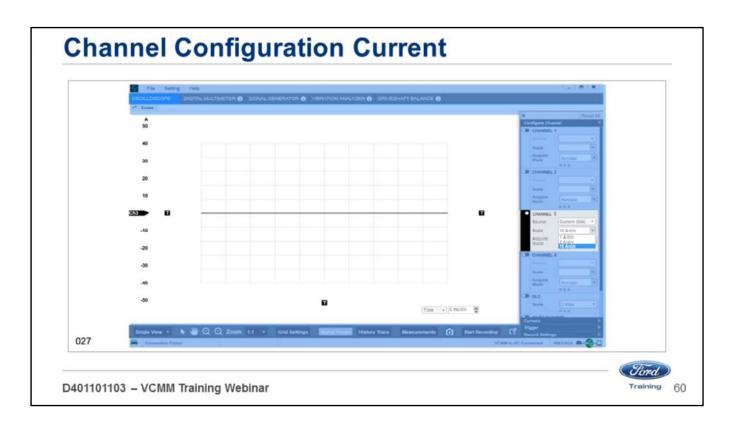
This screen appears when you place one of the current probes in one of the channel ports to test for current flow.
