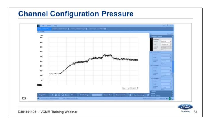
This screen appears when you place the Pressure Vacuum Transducer (PVT) probe in one of the channel ports to test for pressure or vacuum.
