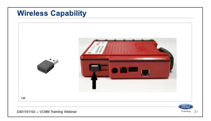
The VCMM ships with two adapters in the kit. These adapters must be installed in the VCMM.
