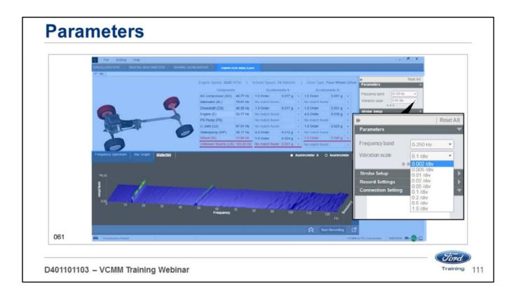
You can change the vibration scale parameters from 0.002/div to 1.0/div.
