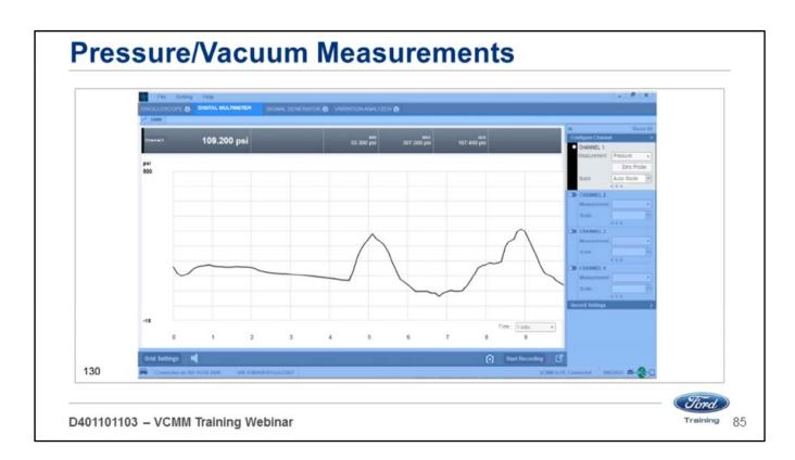
To measure pressure or vacuum place the Pressure Vacuum Transducer (PVT) in one of the four channels:
