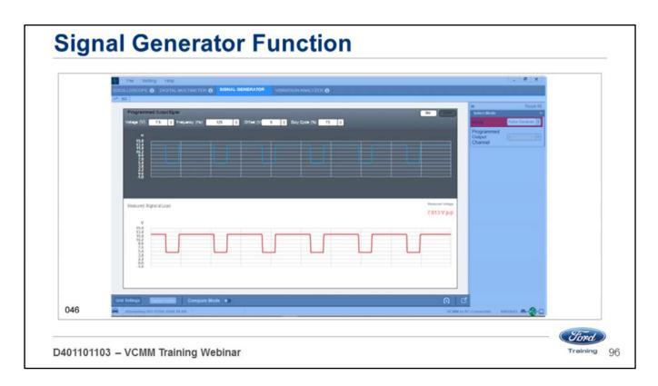
Here is an example of a pulse generator signal at 7.5 volts and 125 hertz with a duty cycle of 73%.
