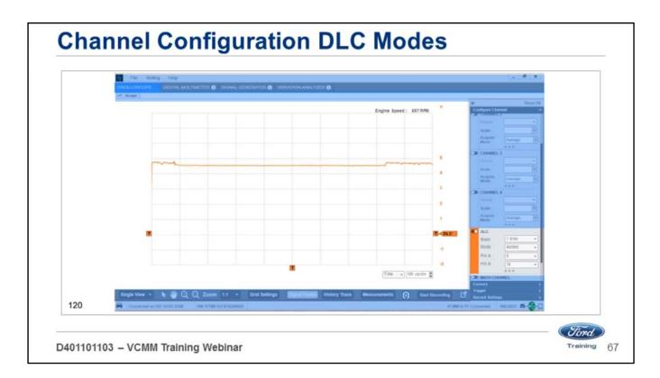
Added mode allows you to monitor the combined voltage of any 2 of the 16 pins in the DLC except pins 4, 5 and 16.
