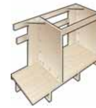
Framed Cabinets (rear view)
