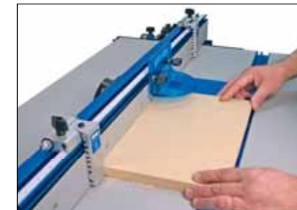
Get extra precision and unmatched repeatability for stop-dados, tenons, etc.
