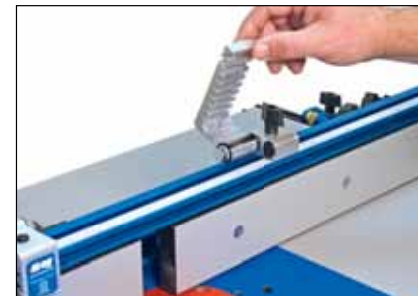
Unique design allows the stop to flip out of the way when not in use.
