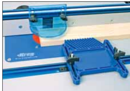
Carefully designed fingers apply optimum pressure to each workpiece.
