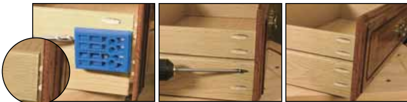
Drill Pocket-Holes at the problem joint.
