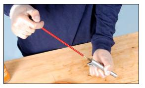
• CLEAN SEMI-AUTOMATIC PISTOL BARREL SEPARATELY WITH SOLVENT
