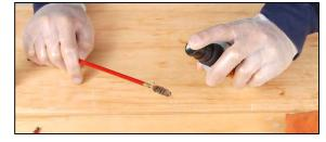
• APPLY CLEANING SOLVENT TO BORE BRUSH (DO NOT DIP BRUSH IN SOLVENT)
