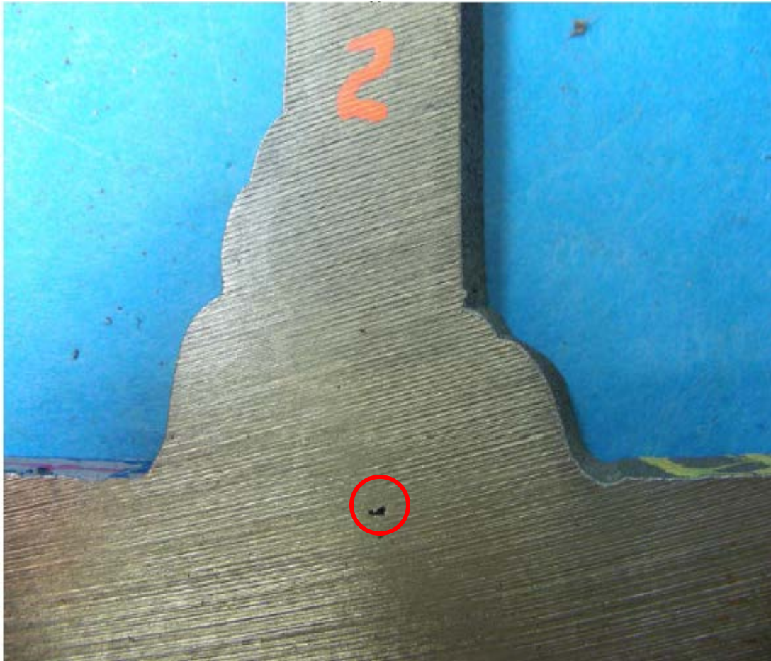
Figure 2. Examination of the cut slices revealed a defect.
