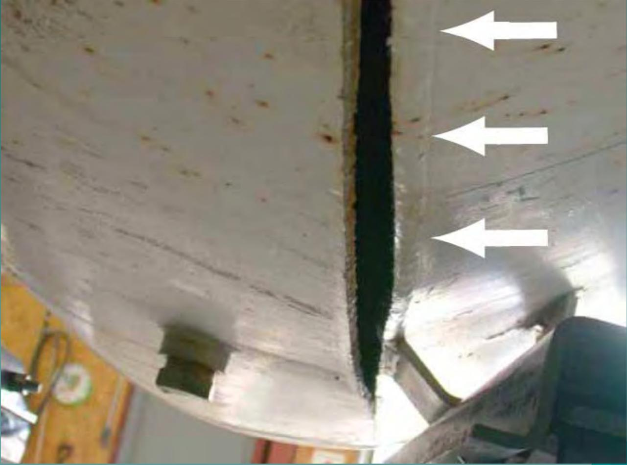
Tank failed hydro test in Canada
