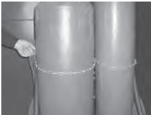
Figure 8: Securing the Cylinders in the Cart
