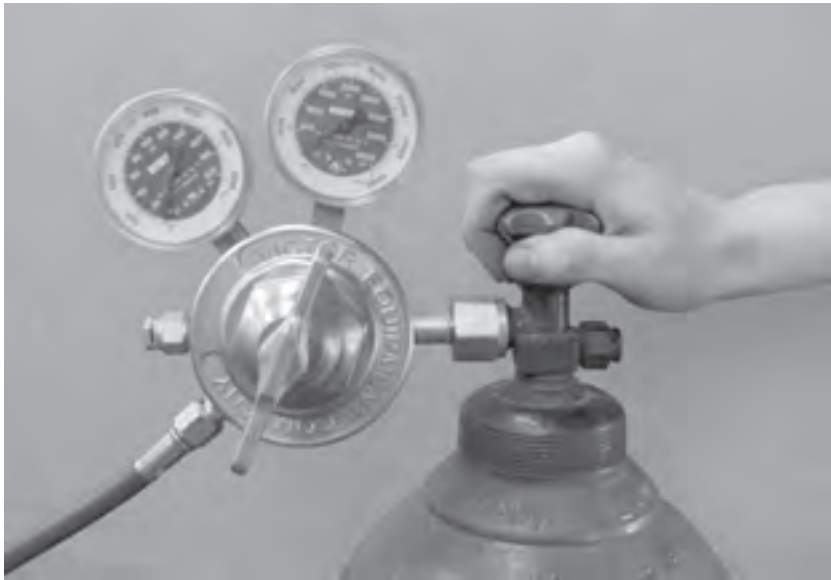
Figure 10: Opening the Cylinder Valve
