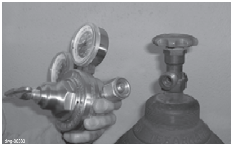
Figure 9: Inspecting the Cylinder and Cylinder Valve
