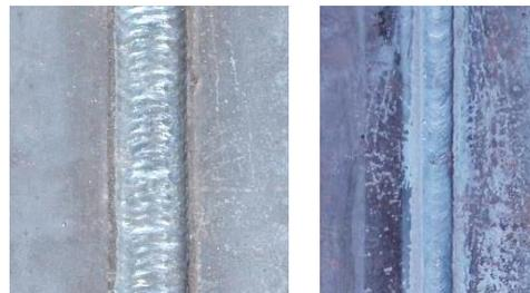
**Figure 7** - Completed welding joint. Left: front side, right: back side of welded joint.
