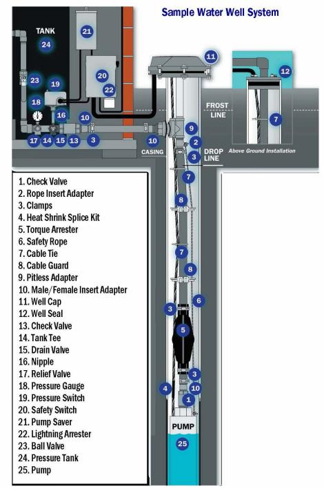
This illustration is intended to demonstrate some of the components that can be included in a water well system and is not intended as an illustration guide. Check local codes for actual requirements and restrictions.
