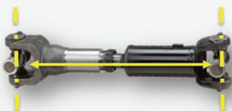
Measure Shaft length from u-joint cap centers
