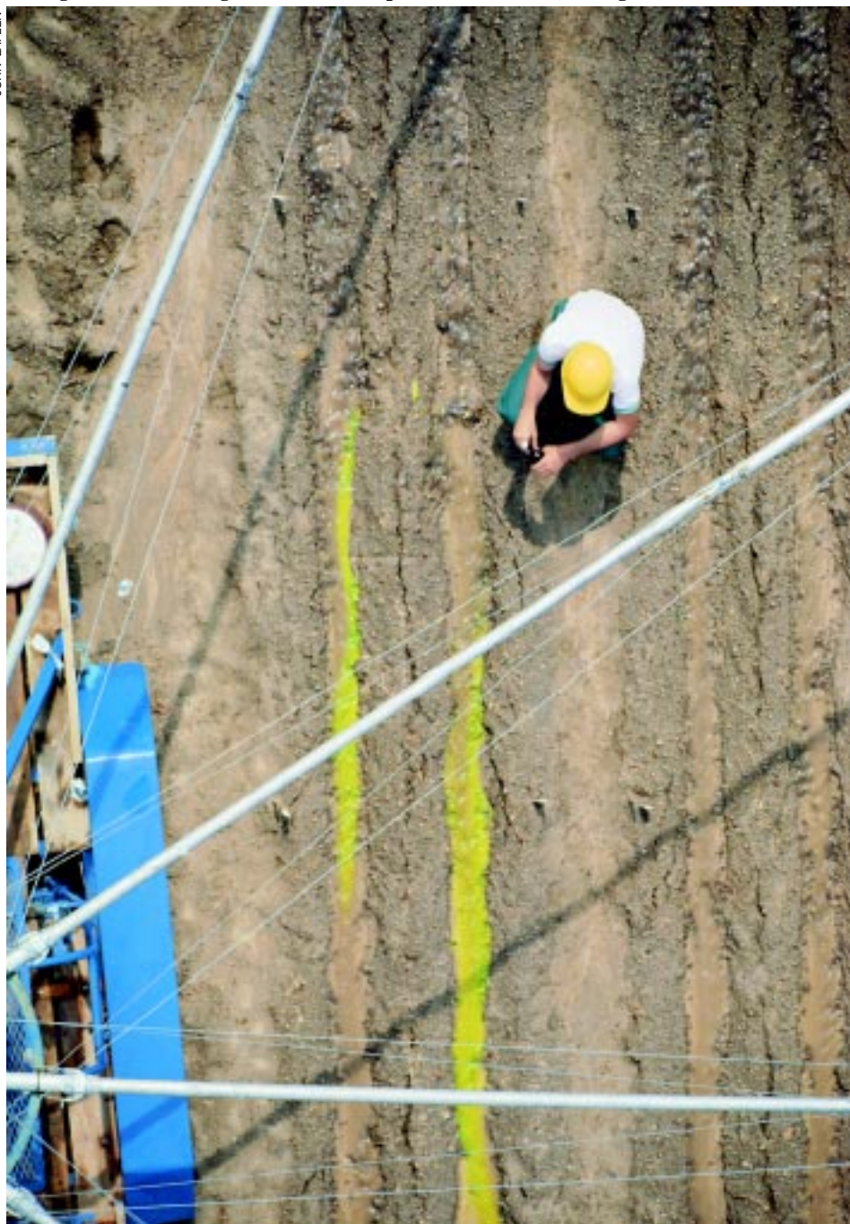
A technician times the rate of advance of a harmless green dye in runoff water coursing through furrows during a WEPP field experiment at Tifton, Georgia.
