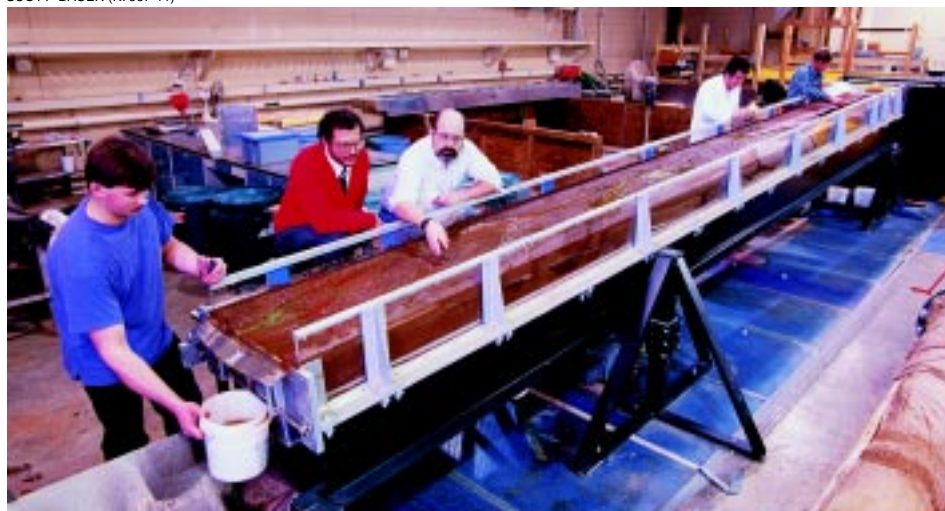
Flume experiments can be used to obtain data on soil detachment and transport by flowing water for use in testing the relationship in WEPP, as well as in development of prediction equations. Here, ARS scientists Mark Nearing (center) and Dennis Flanagan (second from left), graduate assistants Dmitry Bulgakov (left) and Viktor Polyakov (right), and research associate Tingwu Li (second from right) monitor a flume at the National Soil Erosion Research Laboratory.
