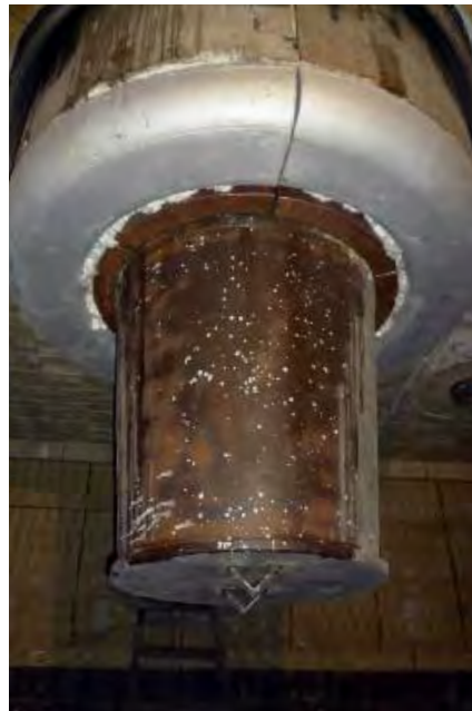
Electrode of a slag cleaning furnace.
