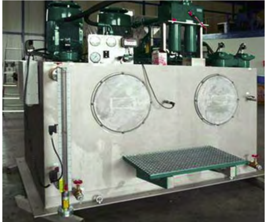
Hydraulic pump station.
