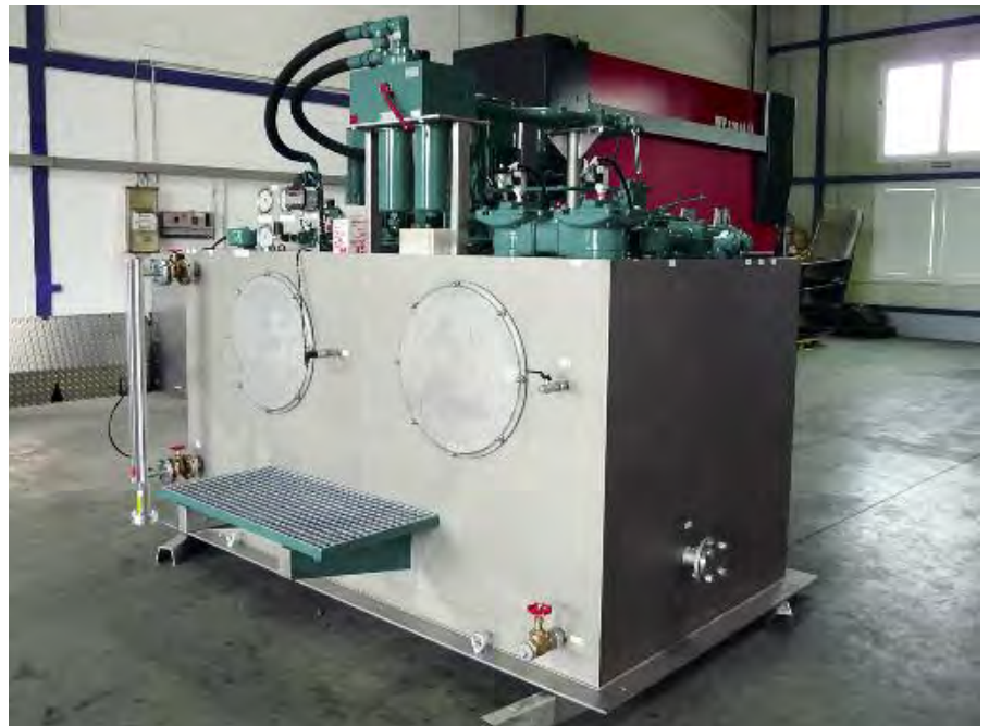
Hydraulic pump station.
