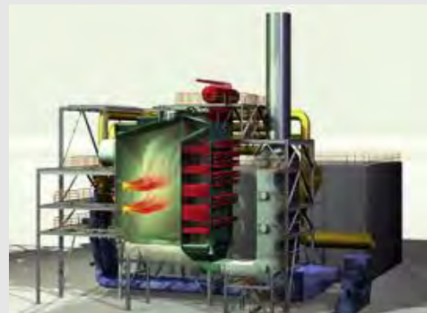
Process gas boiler.
