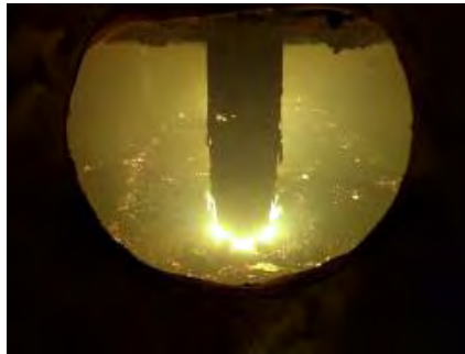
Slag cleaning furnace during operation.
