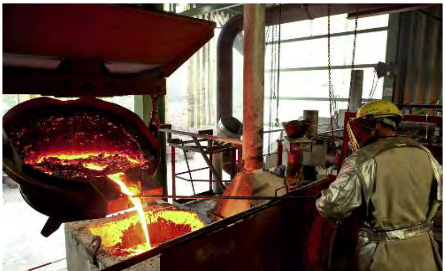
Slag washing machine at Aurubis.
