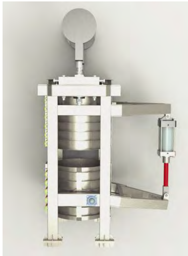
Low cost slipping device for Mini SAF.
