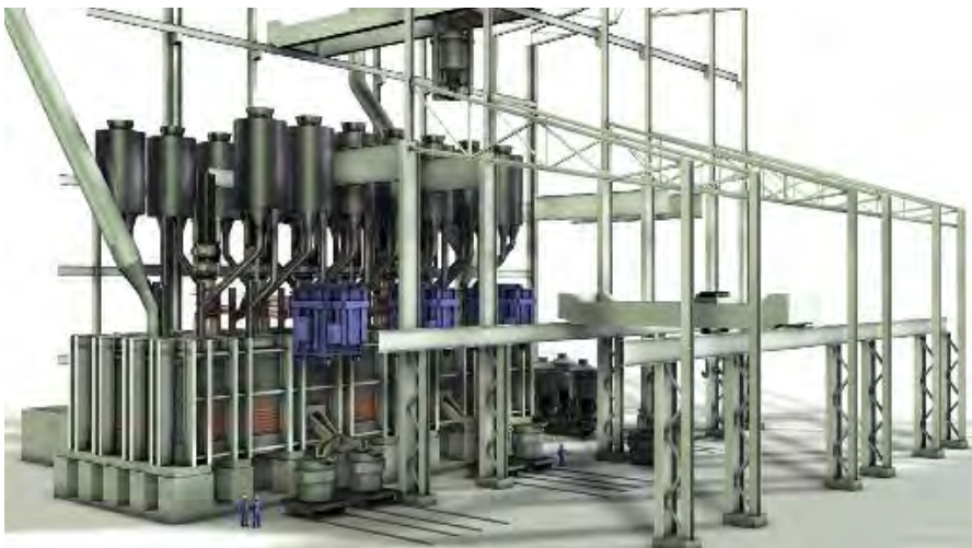
Illustration of the 135 MVA furnace at POSCO SNNC.
