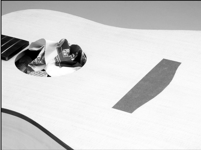
Figure 10. Masked bridge area and blocked sound hole.
