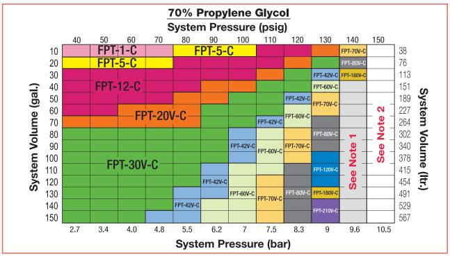
Assumptions: 175 psig (12 bar) Maximum Working Pressure, 100°F (37.7°C) change in temperature, expansion tank precharge 2 psig (0.14 bar) below System Static Pressure.
