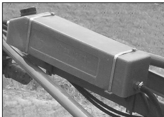
Figure 3.2 Hydraulic Reservoir Installation (2)
