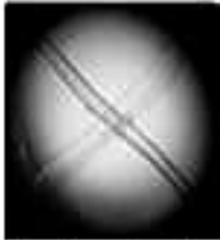
Acrylic - no horizontal lines, vertical extrusion lines, rubs outside fiber
