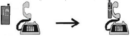
If there is a transmitter in the handset any sounds (pressing buttons, talking, etc) can be heard through the earphone connected to the DD700
