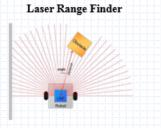
URG-04LX-UG01 is a laser sensor for area scanning. The light source of the sensor is infrared laser of wavelength 785mm with laser class 1 active; Scan area is 240% semicircle with maximum radius 4000mm. Pitch angle is 0.364/ and sensor outputs the distance measured at every point (683 steps). Laser beam diamoters is less than 20mm at 2000mm with maximum divergence 40mm at 4000mm.
