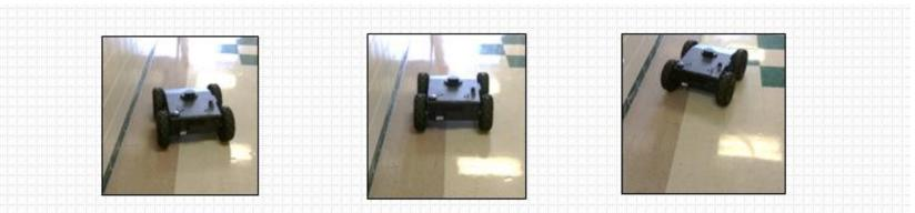
Shown here is the Jaguar 4x4 Robot performing a veerRight behavior to avoid collision with the wall.
