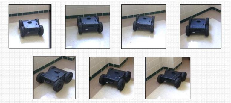
Shown here is the robot moving toward the wall, stopping, turning until no frontal object is detected, then moving forward again until a new obstacle is detected.
