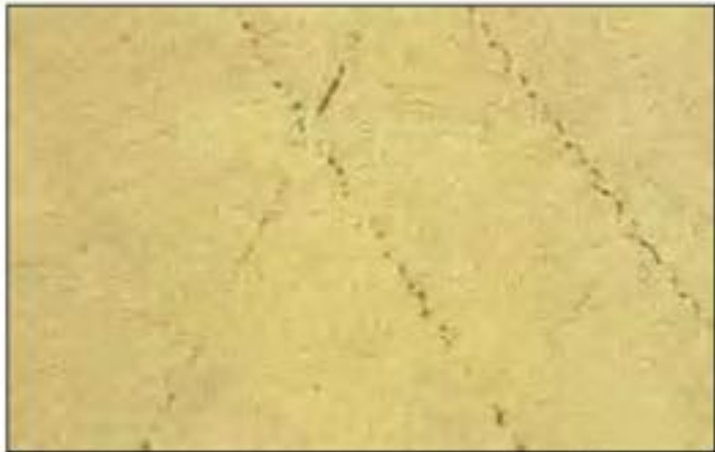
Example: Lapping tracks on Zicalloy, Mag. 200 X.
