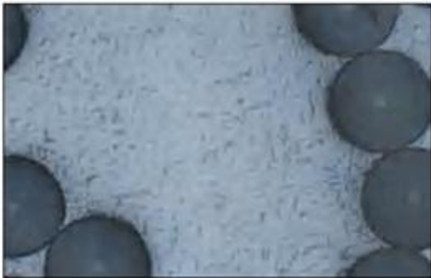
Example: B4C fibres in AlSi, relief between fibres and base material, Mag. 200 X.
