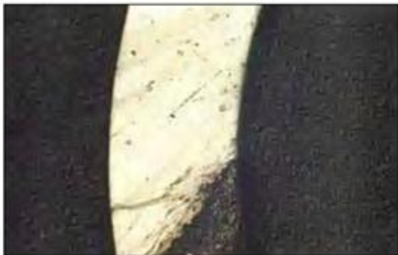
Example: Staining of sample due to gaps between resin and sample, Mag. 20 X.
