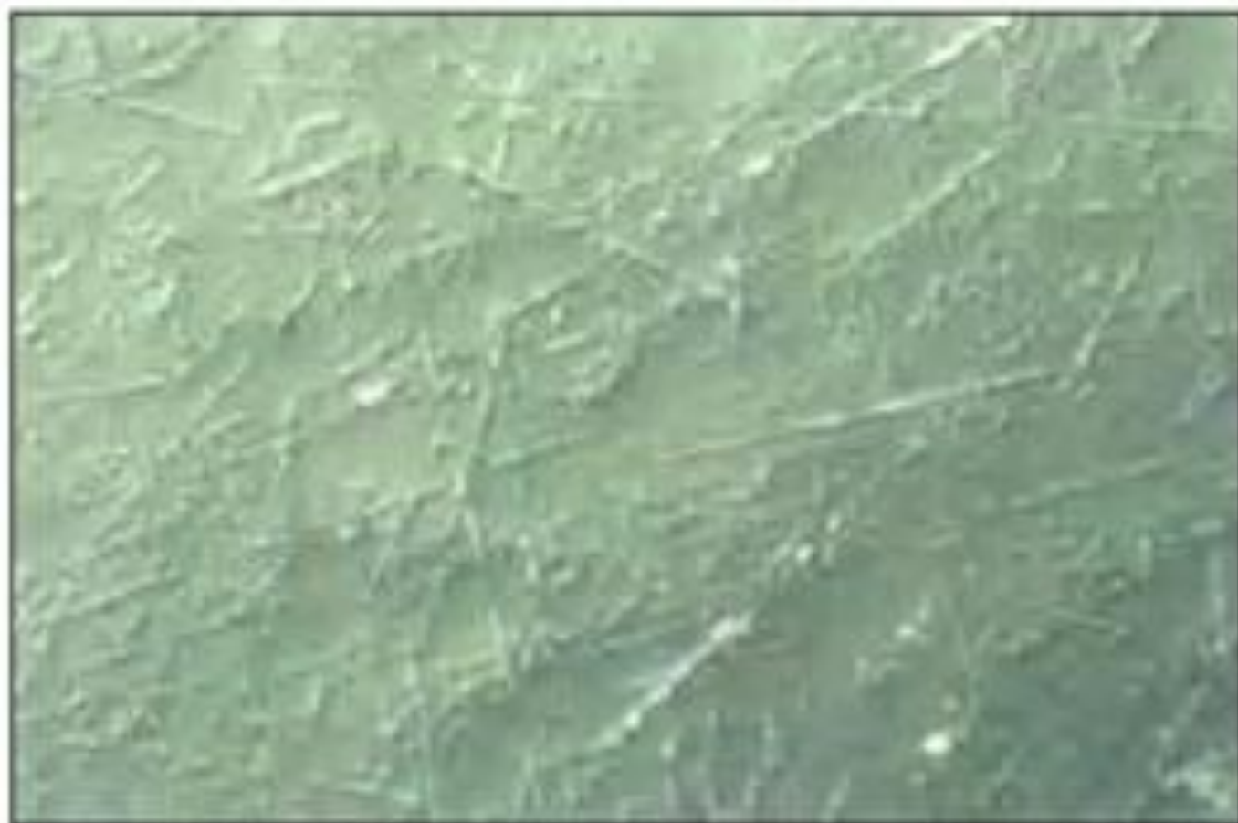
Example: Sharp deformation lines on sample, Mag. 200 X, DIC.
