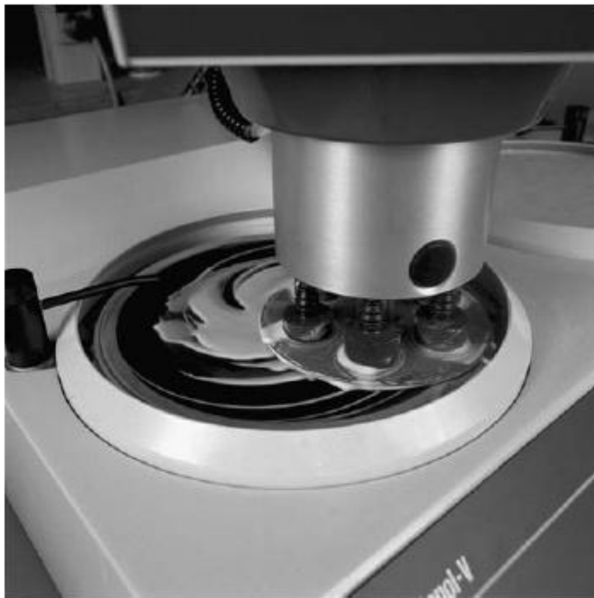
Figure 1.24 Polishing on a rotating wheel with a mechanical sample holder. (Reproduced with permission of Struers A/S.)
