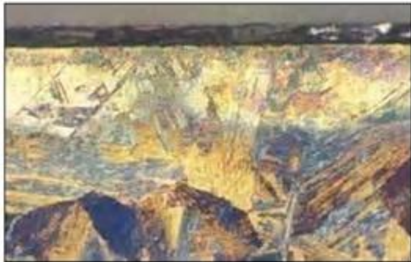
Example: Gap between resin and sample, Mag. 200 X.
