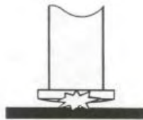
2. Stored energy discharged through weld tip & stud starts downward.
