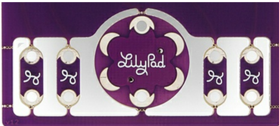
Mouse bites on the LilyPad ProtoSnap allow the PCB to be snapped apart easily.
