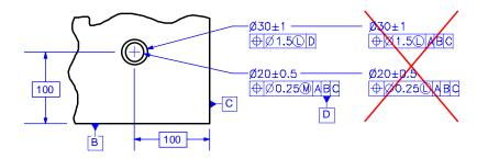
4g. <u>Need to Eliminate the Term "Resultant Condition" [§1.3.51 p.7] and Refine the Term</u> <u>"Virtual Condition" [§1.3.67 p.7] with the Terms "Virtual MM Boundary" and "Virtual LM Boundary".</u>
