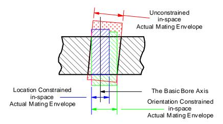
The Actual Mating Envelope concept has two major applications: 1) It is the basis for calculating a tolerance zone size bonus in the presence of the "Geometric Tolerance Value" modifiers (M) and (L). 2) It is the basis for determining the "Actual Mating Size" of a feature based on a size control under the impact of the Envelope Rule.
