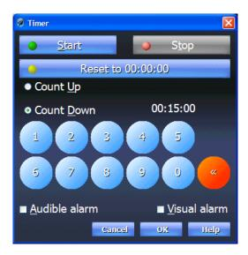
In the timer configuration window, you can also tell the count-down timer to signal when it reaches zero by either an audible alarm (which could be hard to hear in the cockpit) and/or a visual alarm (a message box). Even if neither alarm mode is selected, a count-down timer will turn bright red when it reaches zero. In addition, if the timer is on the Gauge widget (as opposed to the Gaugebar, see Widgets, below), the Gauge widget will come to the front when a timer on it reaches zero.
