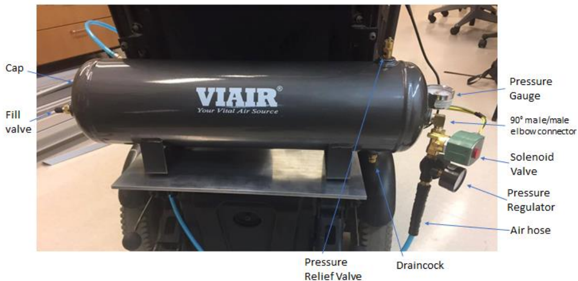
Figure 28: Diagram of setup of storage tank and corresponding valves
