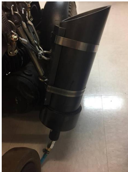
Figure 30: Attached launching tube with air delivery line inserted at quick connect coupler
