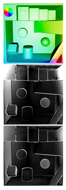
Fig. 7. Left: rendering with optical flow as hsv color overlay; Middle: optical flow endpoint error (0-0.2 pixel, higher errors are white) between ground truth and KinectFusion based scene; Right: stereo disparity error (0-1 pixel, higher errors are white) between ground truth and KinectFusion based scene.
