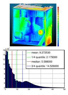
Fig. 5. Targetbox: euclidean error (0-15mm, higher errors in gray), histogram of euclidean errors.
