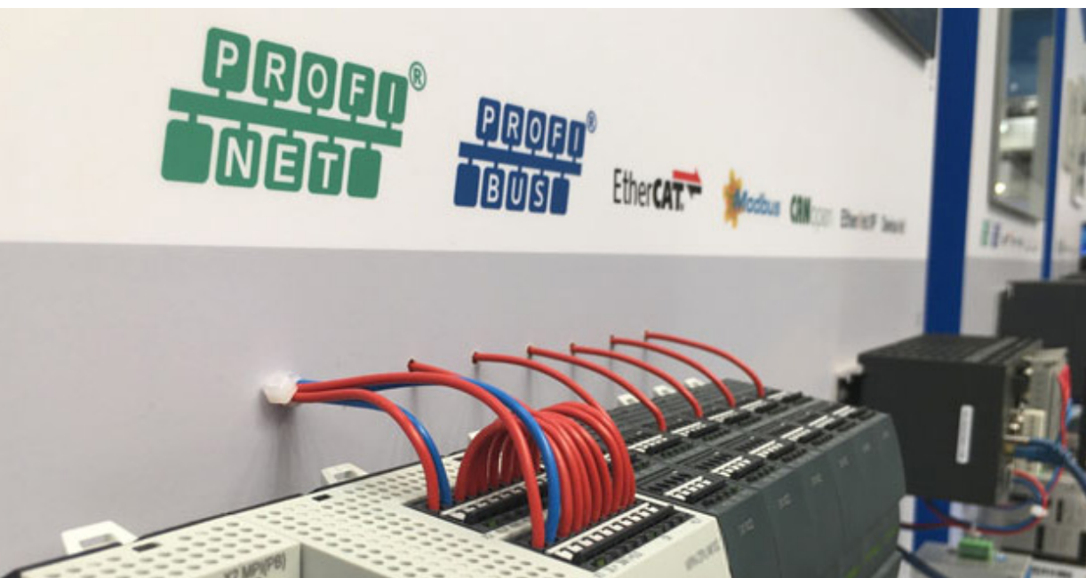
Figure 39. Photo of a demo wall that we took at the 2018 Hannover Messe exhibition floor, showing a list of field protocol logos and test programmable logic controller (PLC) devices at the bottom
