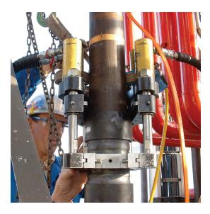
Tool kits are material specific and are available for Brass, Copper, Copper Nickel, Carbon and Stainless Steel pipe/tubing in sizes ranging from 1/4" OD through 3" NPS.
