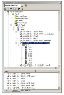
Figure 5 — DeltaV definitions loaded into INS.
