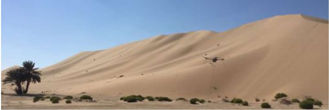
Figure 1. The tethered HARC-TD system provides persistent communications range extension. The product roadmap calls for operation from moving vehicles, >>30 mph winds, and ops at 100+ m AGL.
