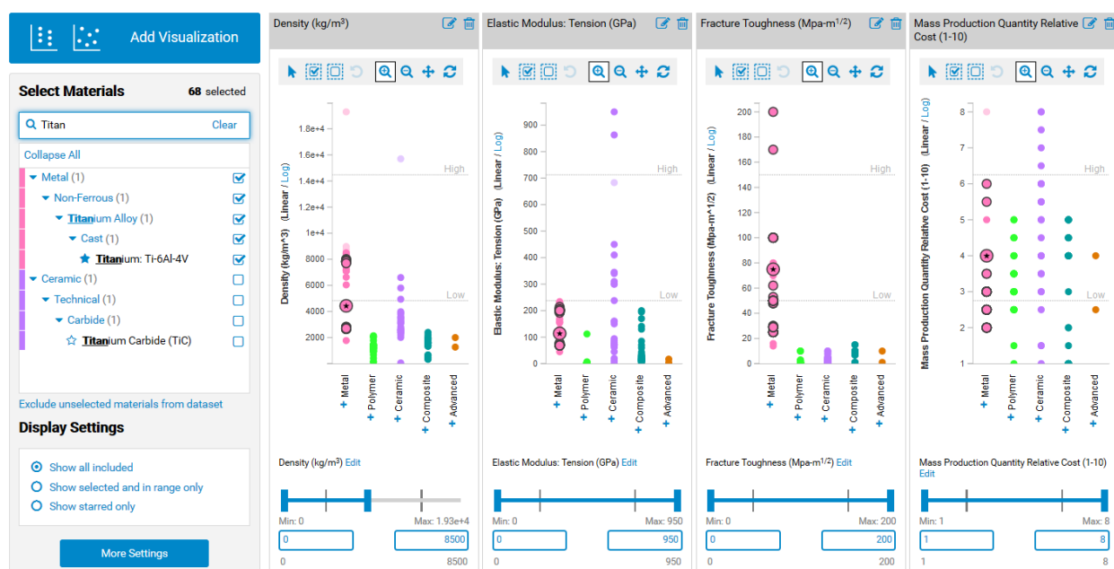
Figure 3: Four linked dot plots, where titanium is selected and starred, and steels and magnesium alloys are also selected. A range filter specifies that only materials with density less than 8500 are “in-range.”
