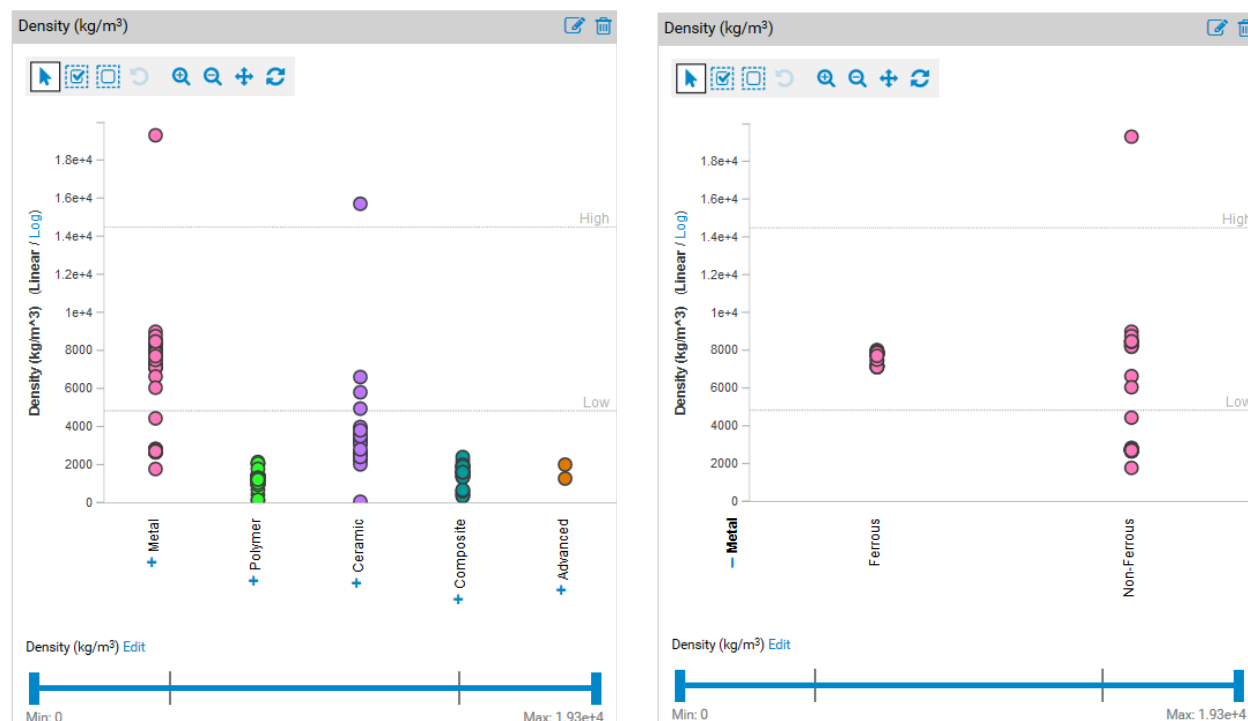
Figure 1: (a) Dot plot of density values for the major material categories; (b) the metal category expanded into its subcategories.
