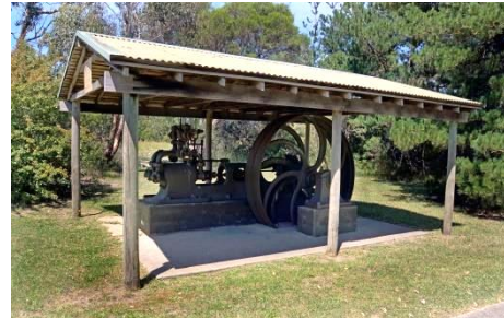
Werner Compressor in Jack Babington Park. From the Somerville Cool Store, this was preserved by the Western Port Lions Club. It was used for the cold storage of fruit until 1970 when the cool store ceased operation
