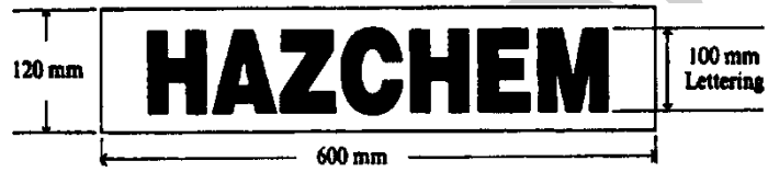
Figure 2 — Template for a placard for dangerous goods (other than combustible liquids) in bulk
