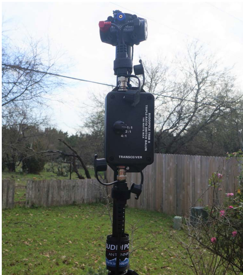
TRSB Triple-Ratio Switch Balun
