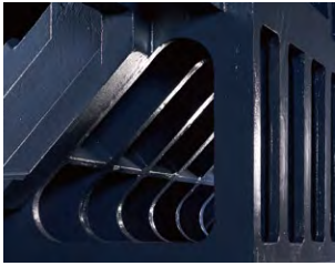
Thick ribs imparting high rigidity
