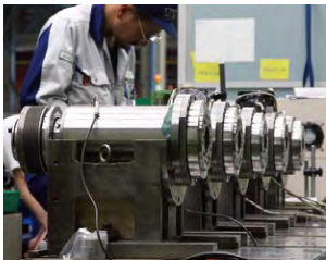
Test running under strict temperature control
